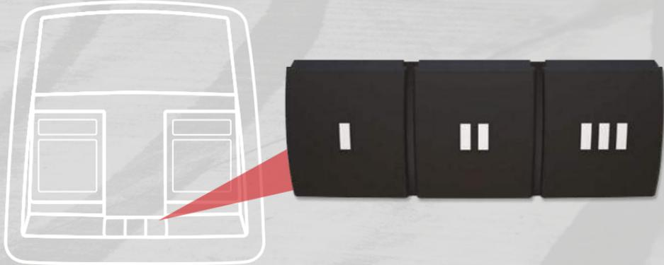
**1** While the car is ON, hold the handheld garage door transmitter 1-3 inches from the HomeLink® button you want to program in the vehicle.
